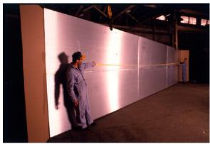
Tank shell for the food processing industry made into one continuous piece using automatic splice welding prior to rolling.
