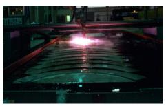
Computerized automatic plasma cutting creates multiple parts and complex shapes up to 3" thick and as large as 96" x 240".
