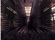
Heat exchanger partially loaded with tubes.
