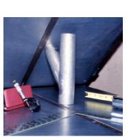
Angle standard being used to check the geometric accuracy of prefabricated piping items.
