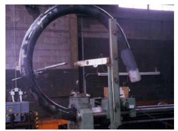
A pines Roto-Bender bends pipe from 5" to 12" sizes and has the capability of producing wrinkle-free bends with the centerline radius as small as three times the outside diameter of the pipe.
