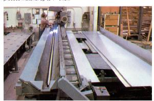
Splice welding using automatic double-sided gas tungsten-arc welding.
