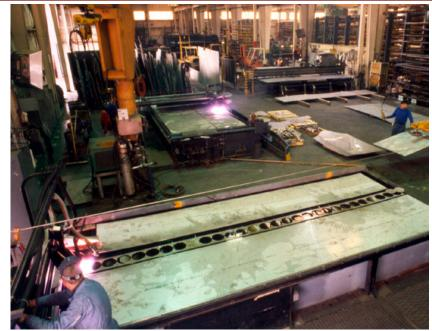
$70 \, \text{ft.}$  wide clear span plate fabrication facility served by overhead cranes totaling  $30 \, \text{tons}$  of lifting capacity.
