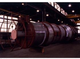
Stainless steel and titanium heat exchanger.
