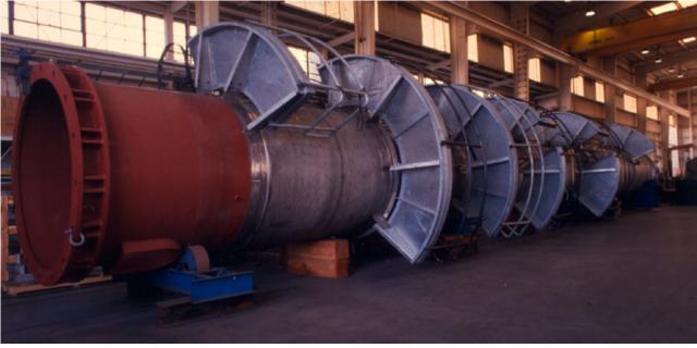
Extractor tower, 90" diameter x 1/2" wall x 83 ft. high with prefit platforms, fabricated from Type 304 stainless steel for the petrochemical industry.
