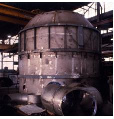
Vapor recompression evaporator sump used in the wastewater treatment industry.
