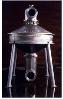
Aluminum wet pump pressure vessel used to transfer fish from a ship's hold to the dock.
