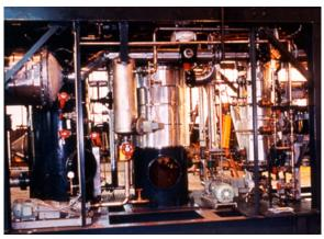
Skid-mounted formaldehyde production plant for the chemical industry completely assembled within our fabrication facility.
