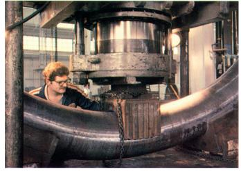
A vertical hydraulic press used to end large diameter pipe in sizes from  $4^{\prime\prime}$  OD through  $24^{\prime\prime}$  OD.
