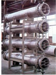
Nickel 200 8-pass, 4-shell heat exchanger.
