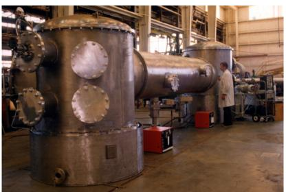
Stainless steel vacuum chamber used for free-electron laser experimentation.
