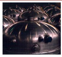
Aluminim hydraulic tanks used in hydrofoil boats.
