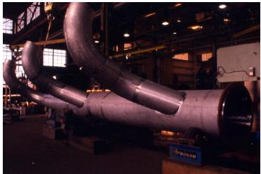
Piping header with polished internal surfaces.
