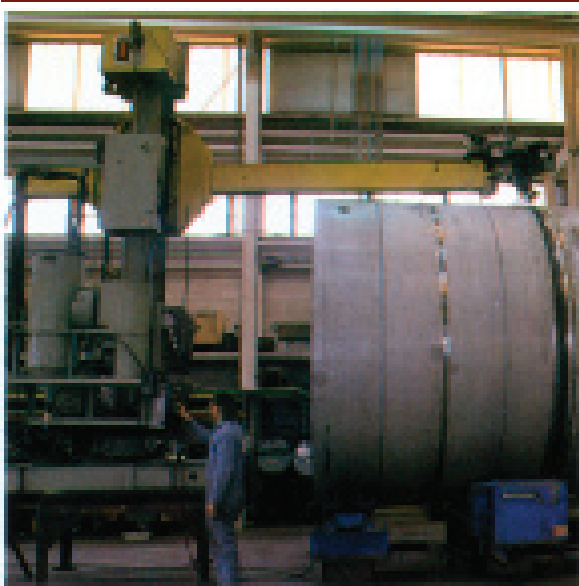
Circumferential seam welding of a large pressure vessel using a submerged-arc welding manipulator and turning rolls.
