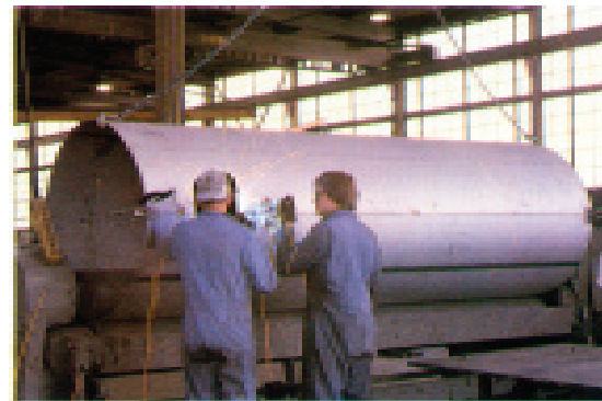
Shell rolling operation can fabricate shells up to 20 ft. diameter and 1/2" thick.
