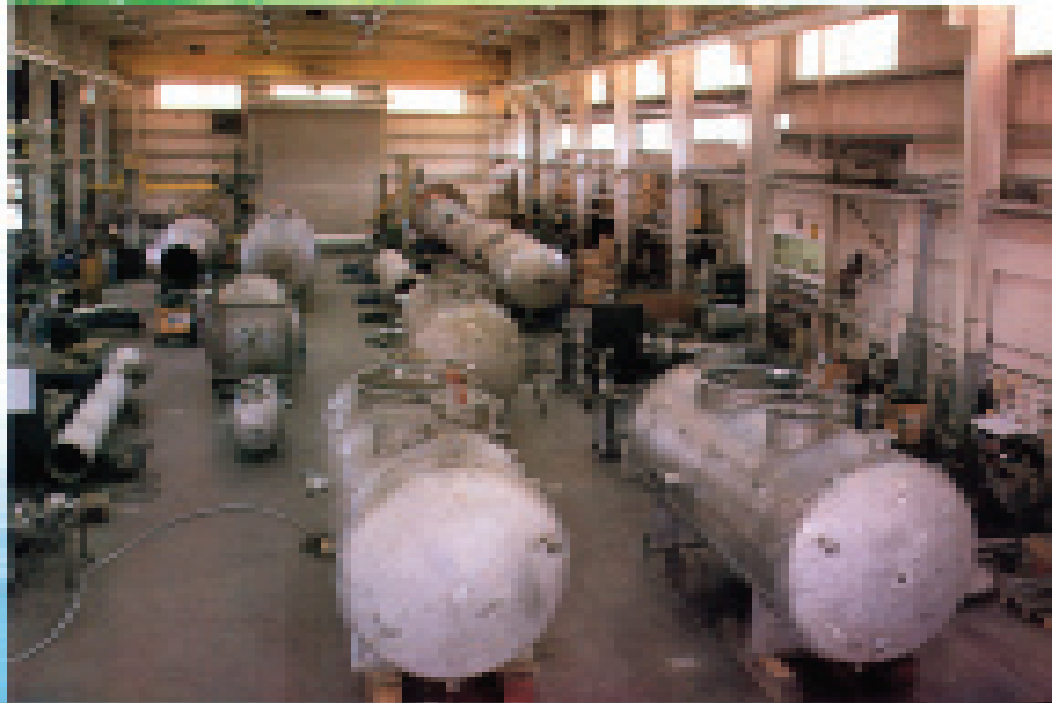
60 ft. wide x 240 ft. long main fabrication bay serviced by overhead cranes totaling 40 tons of lifting capacity with 31 ft. clearance under the hook.
