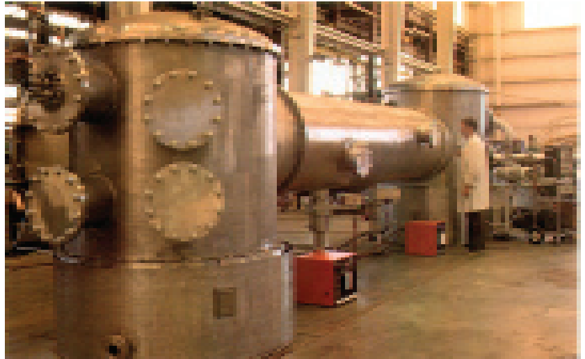
Stainless steel vacuum chamber used for free-electron laser experimentation.
