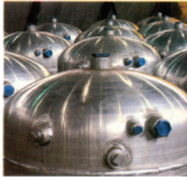
Aluminum hydraulic tanks used in hydrofoil boats.
