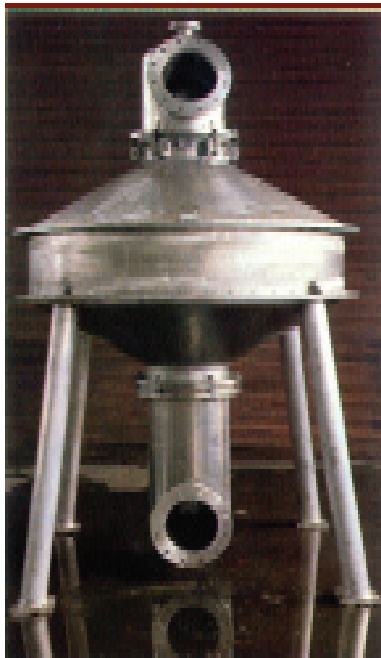
Aluminum wet pump pressure vessel used to transfer fish from a ship's hold to the dock.
