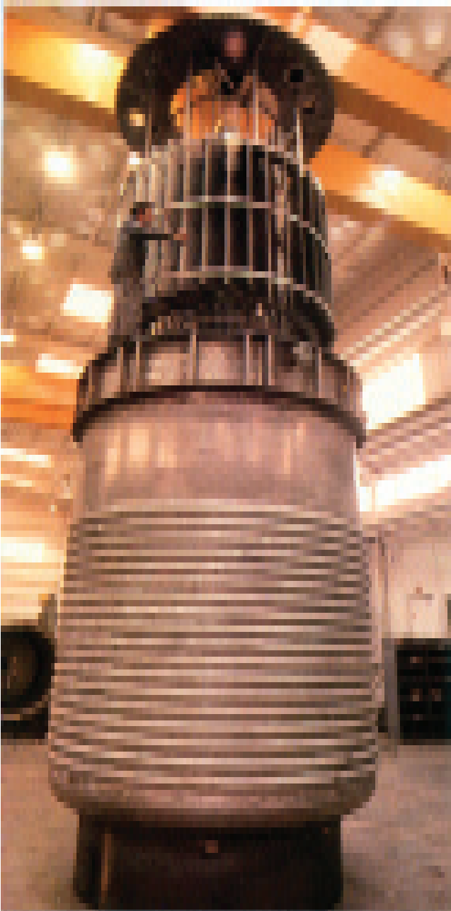
Stainless steel primary slurry tank used for producing plastics.
