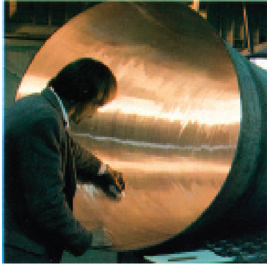
Cotton-test finish on a section of a paper mill headbox piping system.
