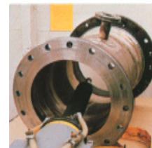
Radiographic inspection checks the integrity of welds.
